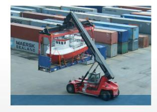
• Flat rack or platform containers are suitable for heavy loads and cargo that need loading from the top or sides (i.e., machinery, pipes, or other bulky items). Flat racks have collapsible walls at the end, while platform containers do not.
